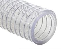
NON-TOXIC FDA / USDA COMPLIANT PVC MATERIAL EMBEDDED WIRE HELIX (SMOOTH TUBE AND COVER) INCREASED VACUUM RATING & CRUSH RESISTANCE CAN BE ASSEMBLED WITH FULL ROLL PURCHASE +25 TO +150 (DEG F) SERVICE TEMPERATURE
